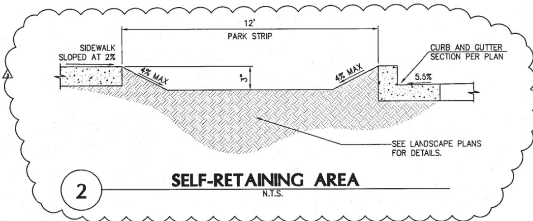
Figure 4-5: Example Self-Retaining Landscaped Area Cross Section
