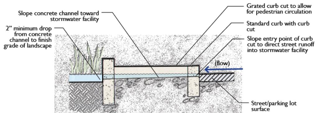
Figure 5-12: Grated curb cut: section view (Source: SMCWPPP 2009)
