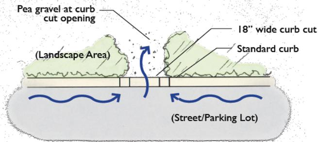
Figure 5-4: Standard curb cut: plan view (Source: SMCWPPP 2009)
