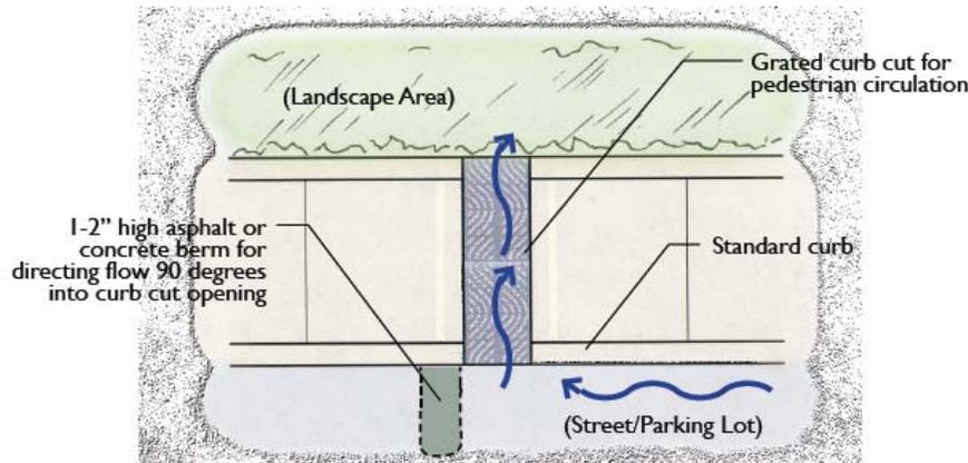
Figure 5-13: Grated curb cut: plan view (Source: SMCWPPP 2009)
